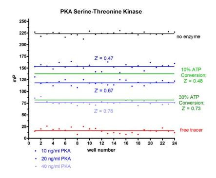
A robust ADP-detection module leads to a robust Transcreener<sup>TM</sup> Kinase Assay. Kinase reactions containing 10  $\mu$ M ATP and 10-40 ng/mL PKA were incubated for one hour at 25°C as described in the Materials and Methods. The resulting Z' values demonstrate a high quality kinase assay at low % ATP conversion. Lines represent the means of the 24 data points. The green lines correspond to 10% and 30% ATP conversion.
