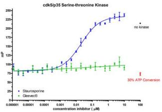
Dose-dependant inhibitor curves confirm the potency of Staurosporine and Gleevac® towards PKA, cdk5/p35 and Abl. Kinases (at similar concentrations as those used in Fig. 6) were incubated with two-fold serial dilutions of Staurosporine and Gleevec® in the Transcreener™ Kinase Assay. The corresponding IC50 values for Staurosporine were 0.5 nM for PKA, 20 nM for cdk5/p35 and 47 nM for Abl. Gleevec® only inhibited the tyrosine kinase Abl; IC50=69 nM.
